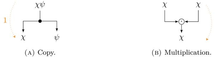
FIGURE 1. Propagation rules for copy and multiplication operations.
